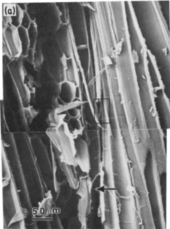
Figure 5 (a) The zone of the crack tip shown in Fig. 3. (b) Higher magnification of a zone in front of the crack tip in (a), showing splitting of a cell wall.
